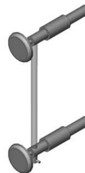
Figure 6.4: Gauge Glass Installation
